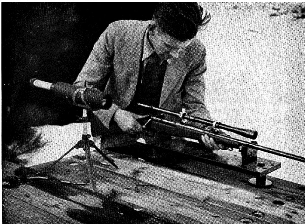
A machine rest mounted on a sturdy shooting bench is excellent for testing your ammunition, the Weaver rest is quite inexpensive but highly efficient
