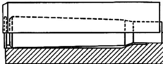
A useful headspace gauge for determining the headspace or mechanical requirements of a Springfield rifle case. This gauge is made by L. E. Wilson, of Cashmere, Washington. In using it one merely drops the properly resized case into a special chamber manufactured to exact case length. There are steps on each end indicating maximum and minimum. If it projects above the maximum at the head, the cartridge case has too much headspace. If it drops below the step, too little. On the opposite end, if it projects beyond the high step, the case is too long, and needs trimming. If below the low step, it is too short, although it can be used if it meets other requirements
