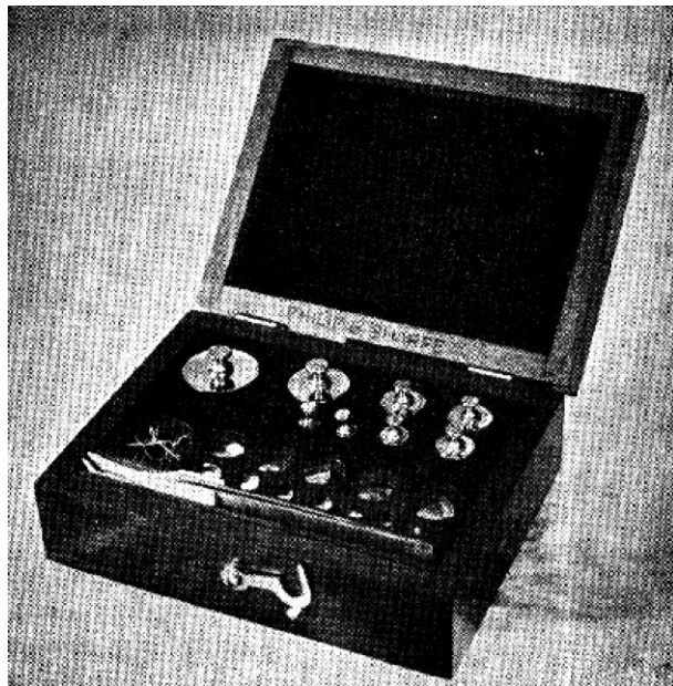
The author's set of master weights, made by Voland & Sons to Class S Bureau of Standards specifications.
