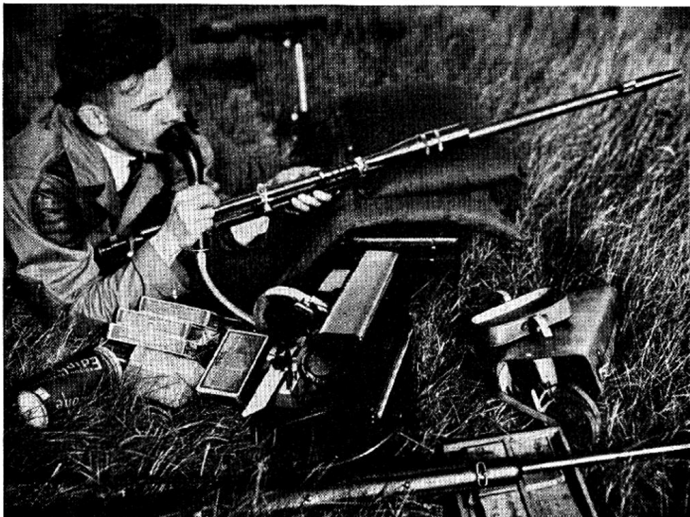
Comfort on the range. A new version of recording firing data by means of a dictaphone. The author's dictating machine fitted with a six-volt motor (used with transformer on 110-volt circuit) is run with a sixty-foot cable from the auto battery. Report of each shot is made at time of firing, giving full details on light, wind, load and other pertinent facts. This system of recording is used by the author in his routine test work
