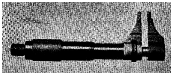
Inside micrometers are extremely useful for gauging neck diameters. Minimum diameter possible with this unit is \cdot200 inch
